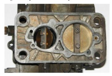
butterfly does not start to open until the (smaller) primary choke butterfly is about half open as in the photo on the left. If the secondary butterfly is opening too early, there's a problem with the linkages connecting the two butterflies.
