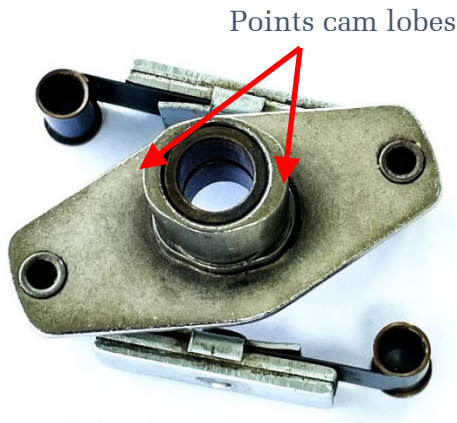
Photo 4 Points cam, springs and centrifugal weights looking from the front, ready for fitting onto camshaft. Note how the springs are fitted.
