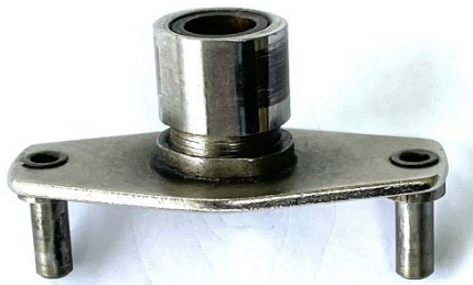
Photo 1. Points cam with centrifugal weight pivots
