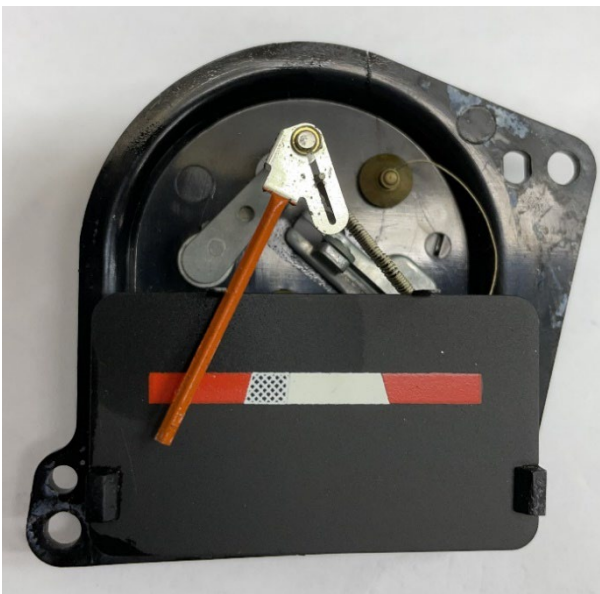
Photo 6. Front of Battery Meter
