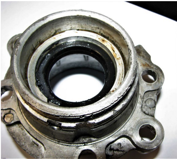
Photo 19: Shows the output hub oil seal of size 31x42x8 mm. Fitted from the outer end of the hub (upper-most opening in the photo). The open side of the seal (with the rubber lip and spring) faces downwards in the photo, i.e. towards the gearbox.
