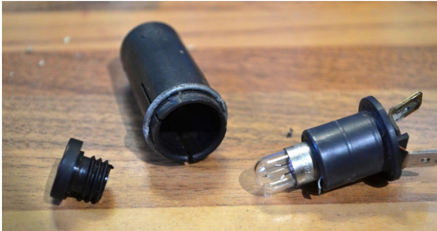
Fig. 10 2CV instrument panel light assembly. Note the spade connectors at far right.
