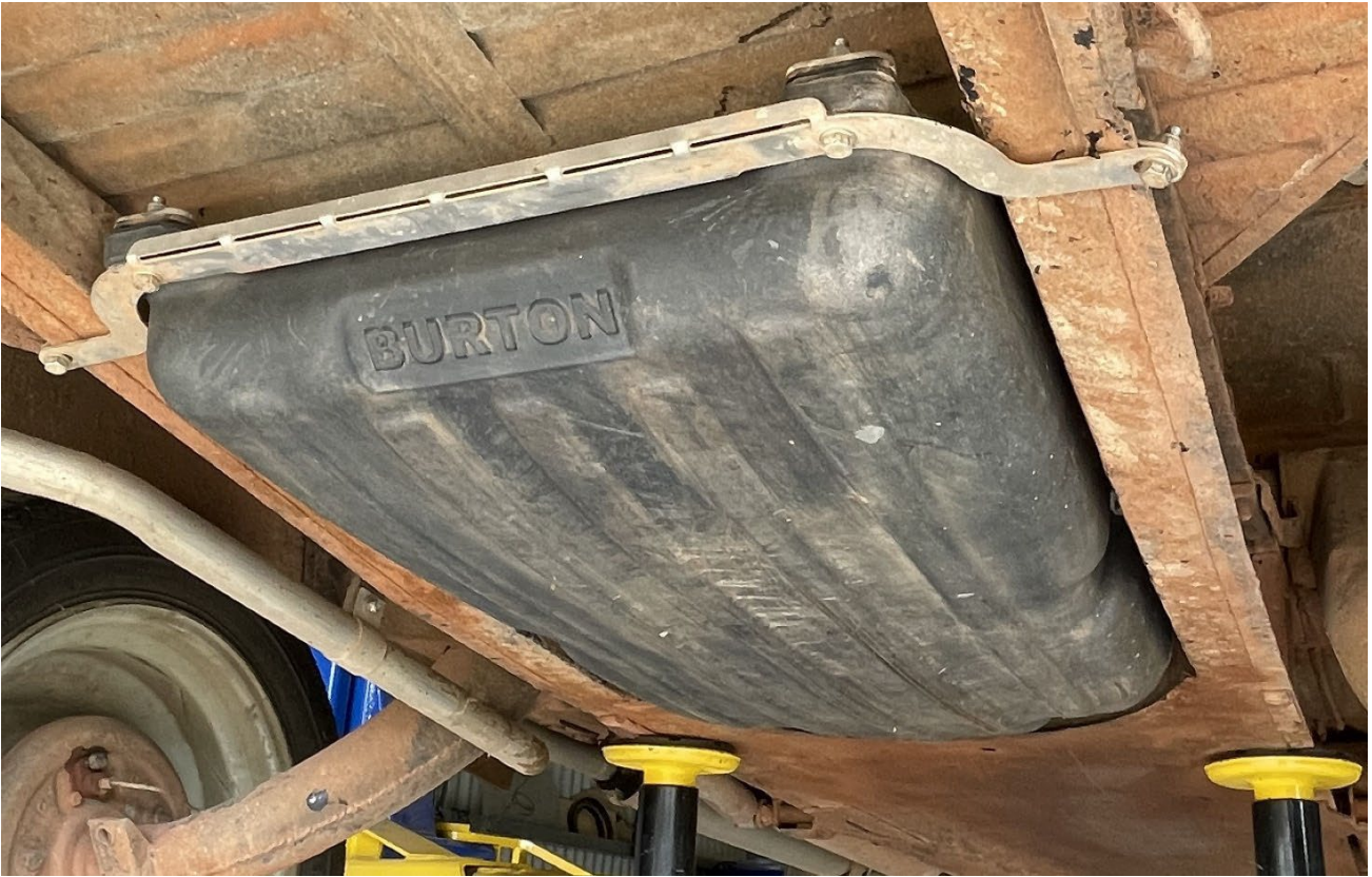
Fig. 2 The 40-litre fuel tank in-situ, in the company of some left-over Red Centre dust! Also shown is the tank's rear mounting bracket (supplied with the tank).
