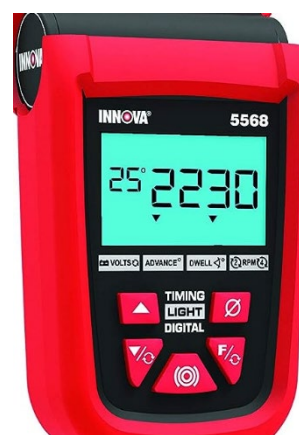
Fig. 1-3. Control panel showing 25° of advance at 2230 RPM.
