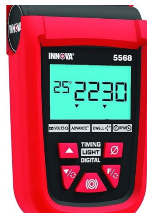
Fig. 1-3. Control panel showing 25° of advance at 2230 RPM.
