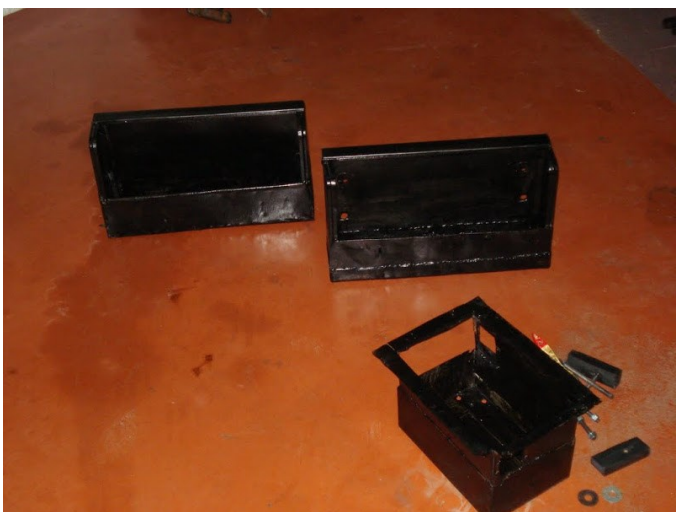
One of the two "toolbox" compartments, as they are in the bottom of the car, they are very vulnerable; this one was hit by something during the 84 years of life of this car. The most complicated part (and visible when fitted on the car) was in good shape; all the bottom part was built from scratch.
