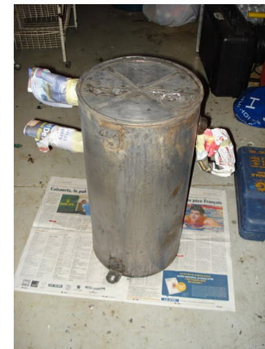
Fuel tank stripped and ready to be painted: the fuel tank is just atop the engine: no fuel pump; gravity does the job.
