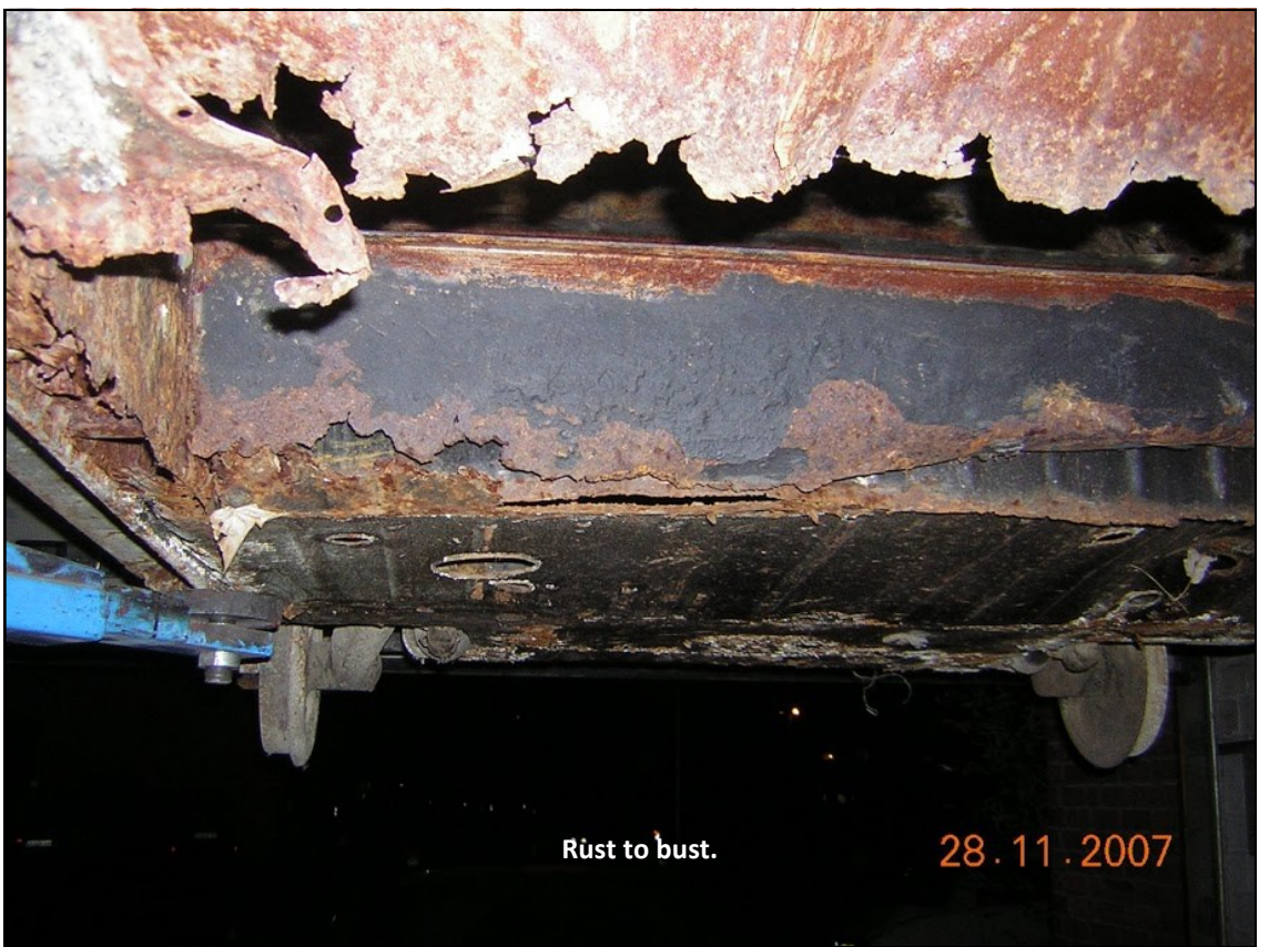
The car has been parked outside 28 years, without hood, wingless, the hood is open ... all the mechanics and hydraulics were destroyed by rust.
