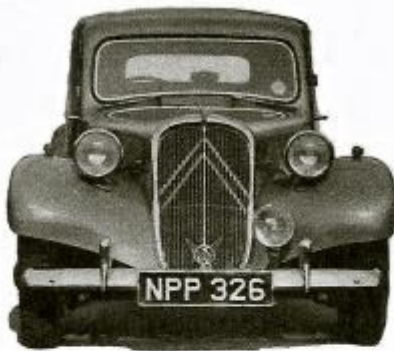
The Citroën chevron motif is attached to the rear of the radiator grille, and a small detachable plated pressing covers the hole in the bottom of the grille that accommodates the starting handle. The fog lamp is an extra fitting.
