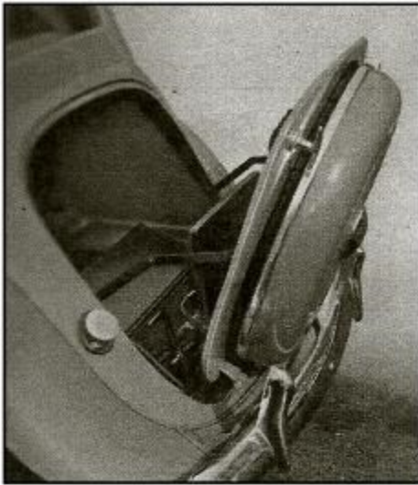
The spare wheel, carried on the outside of the luggage locker, is protected by a cover released from inside the lid. Tools are carried in a detachable box that fits in the bottom of the luggage compartment. To increase carrying capacity with the locker lid in the open position a hinged flap attached to the inside of the lid can be lowered to form a platform.
