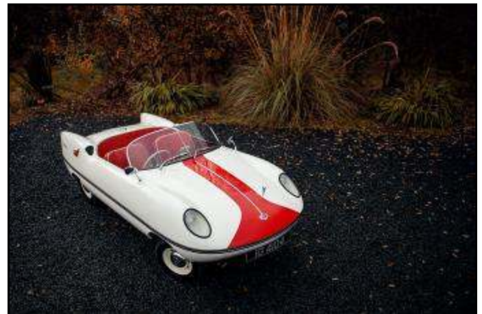
Weighing just 380 kilograms or 840 lbs the tiny Dart is powered by a two-cylinder, two-stroke engine mounted in the rear
