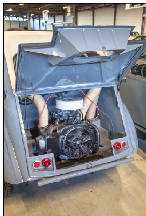
After deciding they needed a four wheel drive for Africa, Citroen developed the 2CV Sahara with two 425cc engines, one in the front and one in the rear, each with separate ignition switches. Only 694 were sold, though production lasted from 1960 to 1966. In 2012 an unrestored Sahara sold in the USA for $(A)185,000.
